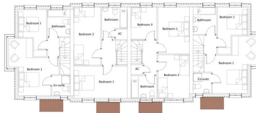
Proposed First Floor Plan - Plot 21, 22, 23 & 24 Scale 1:100 @ A1
